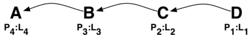
Figure 2: In deepest match, an exact match for each part of the name is looked for. The matching begins from the end of the name (above D) and proceeds a part by part to the beginning (A), until a match or there's nothing to look for.
